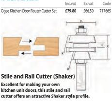
One of the biggest advantages of such cutters is that you have just one cutter for the moulding and scribing cuts. To use, simply alter the height of the cutter in the router table to switch from one operation to the other. The timber should be positioned face down on the table surface for the moulding cuts and face up for the scribing cuts.
