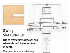
this set includes: 4 x 3 winged cutters 3.2, 4, 4.8, and 6.4mm in width. 1/2" shank arbor. 21 shims (8 x 0.1mm, 4 x 0.5mm, 5 x 1mm, 2 x 3mm and 2 x 6mm). N.B. The carbide edges of the cutters should never touch; arrange the cutters to prevent this. Use only the thicknesses provided in the set. Be sure all cutters are assembled in the correct rotational direction.
