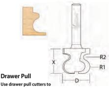
Use drawer pull cutters to create flush fitting cabinet doors and drawers.
