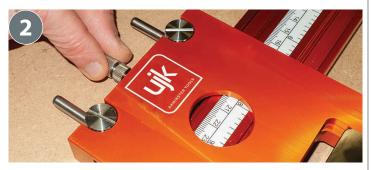
**3.** A lens and a scale with cross hairs (3) allow you to position the jig precisely both in relation to the scale on the Progrip clamp and in relation to a line marked on your workpiece.
