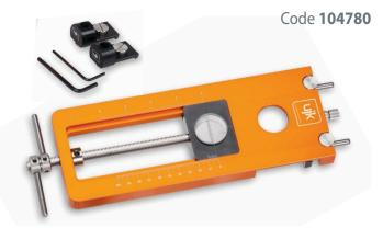
**4.** For greater precision a vernier scale with a micro adjuster (4) allows you to set the jig with an accuracy of 0.1mm. If you wish to cut a groove wider than the cutter, the scale and threaded adjustment provide the necessary control for the second pass. If after the first cut the groove is too narrow, you can always use the micro adjuster to shift it a smidgen for a second pass.
