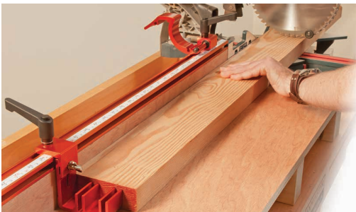
Production stop with adjustable height to suite various back fences
